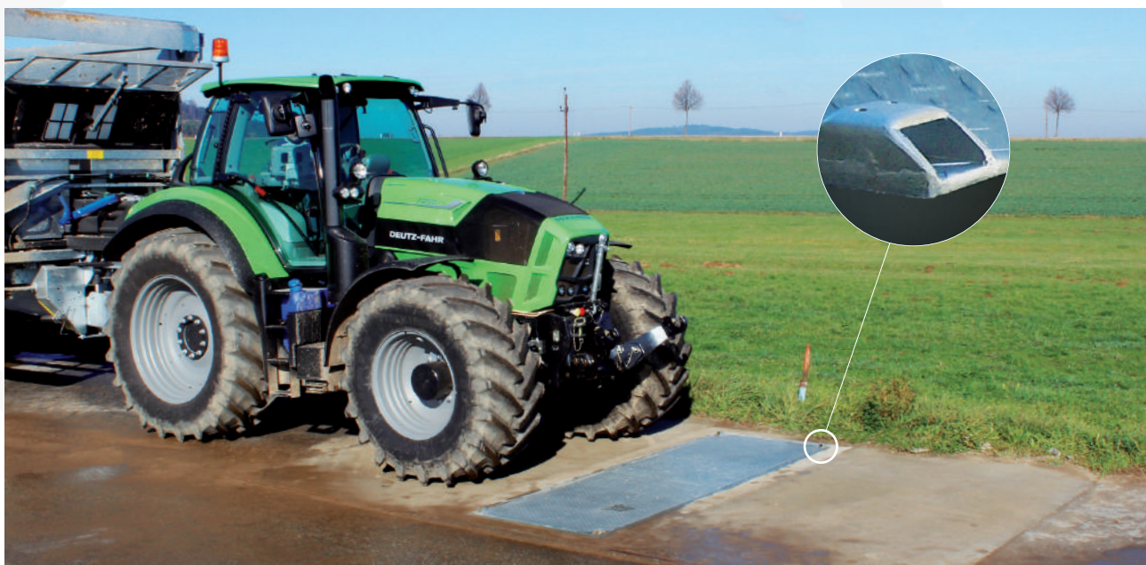
Axle recognition through light barriers.
