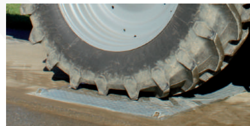
The drive-over-scale also weighs large low pressure tyres.
