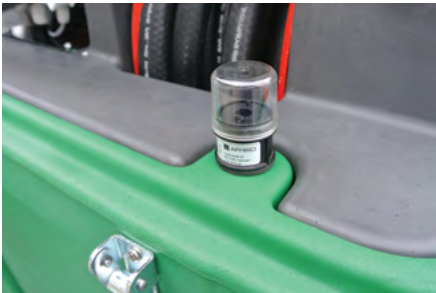
Monitoraggio intercapedine. Leak detector.
